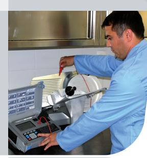
The MI 3310 25A SigmaGT is a multifunctional portable test instrument intended to perform all measurements for complete testing the electrical safety of portable electrical equipment. The instrument can operate from mains power or batteries.
